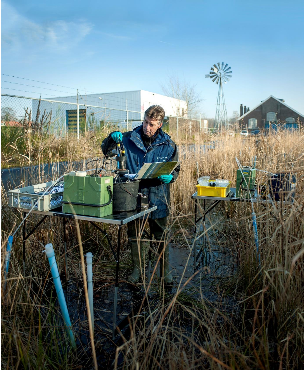
Figure 3: Elaborate monitoring on the Amersfoort site proves that constructed wetlands can purify grey groundwater even in winter. © Deltares/Welmoed Jilderda; featuring field worker André Cinjee
